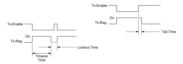
Figure 2.8 T856/857 Transmit Timers
