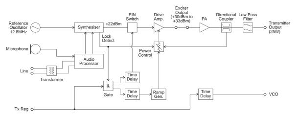
Figure 2.1 T856 High Level Block Diagram
