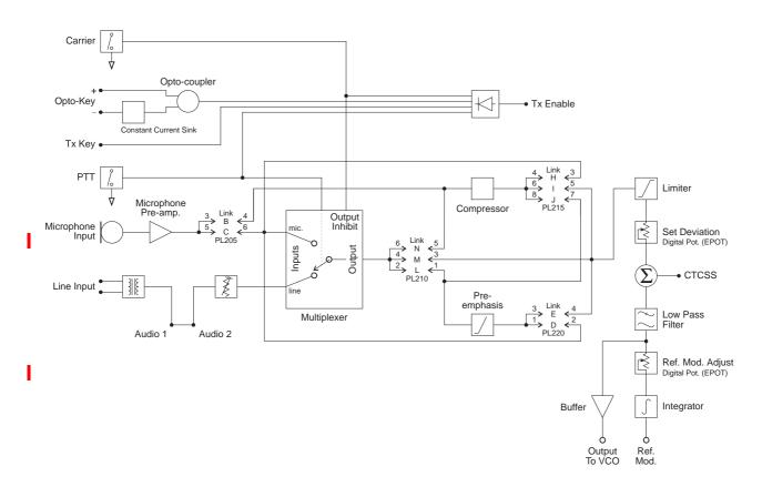
Figure 2.6 T856/857 Audio Processor Block Diagram
