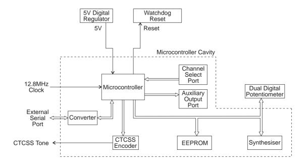
Figure 2.3 T856/857 Microcontroller Block Diagram
