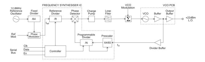
Figure 2.4 T856/857 Synthesiser Block Diagram
