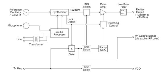
Figure 2.2 T857 High Level Block Diagram
