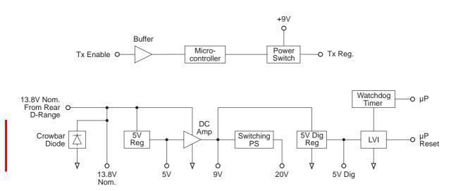
Figure 2.7 T856/857 Power Supply & Regulators Block Diagram
